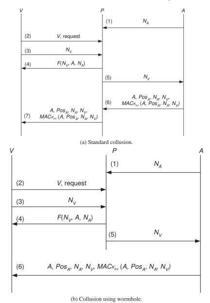
**Fig. 2.** Protocols under Collusion of nodes A and P
